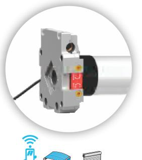
The WSME50 is a remote control version of a mechanical limits motor, with the addition of manual override. This feature allows a roller shutter or awning to be operated by a crank handle in the event of a power failure. The manual override feature is to allow for emergency operation only and is not suitable for general usage.
