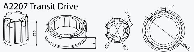
These are adapters to allow connection of our 35mm motor fittings onto a 25mm motor.
