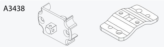
Motor bracket and mounting plate for star head motor only.
