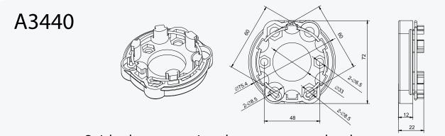
Quick release mounting plate to secure star head motor.
