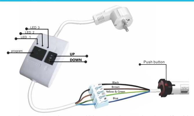
Notes: When UP/Down/Program button is pressed, light LED1 is on. When Program button is pressed for 2s, light LED2 is on. When Program button is pressed for 10s, light LED2 is off and LED3 is on.
