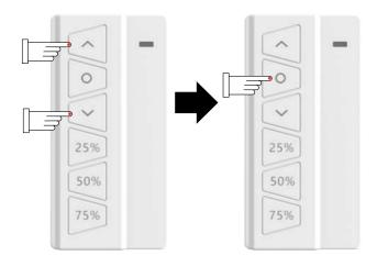
Make the motor at learning state (refer to motor's user manual), press remote's UP and DOWN buttons simultaneously once, then short press STOP button once, the motor vibrates, the remote is paired to the motor.
