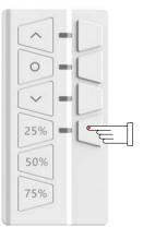
a) During Sleep Mode (all lights are off), press any one switch button once, could check which channel have been set (corresponding light will shine).
