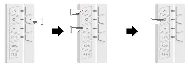
Short press the Channel Switch Button to select a channel (from 1 to 4), once selected, the corresponding light will shine.
