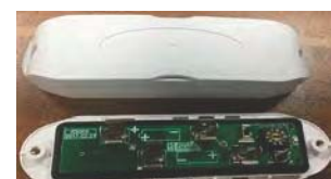
Lift outer cover from circuit board
