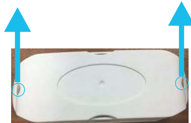
Remove two screws by screwdriver
