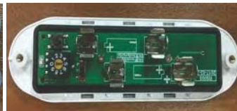
Circuit Board Contains clips onto the mounting base
