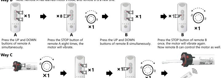
Press motor head's button for 1s till the motor vibrates
