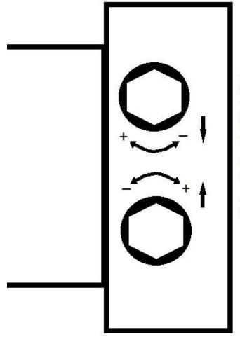
Rotate the limit adjustments to increase or reduce the distance the motor will travel in the direction of the arrows on the right.
