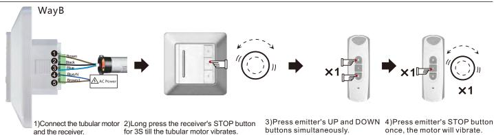
4 Copy Note: Emitter B can control the tubular motor after it learns code from emitter A
